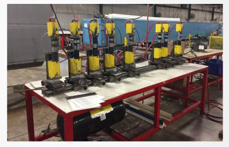
important to all manufacturers, particularly small and general industry shops, where feed drills are a great fit. These shops need tools that offer a small footprint and are reliable and durable. Programmable feed drills offer the ability to customize machining processes with the specific speed and torque needed for a company's particular applications and materials, while providing quality control without variables. The last thing a manufacturing shop needs is lost productivity.
